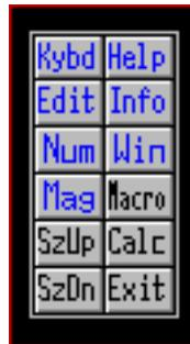
The Control panel allows you to open and close all My-T-Soft TS panels. Click on each key to perform the toggle action. Blue (highlighted) letters indicate an open panel, black letters indicate a closed panel.
