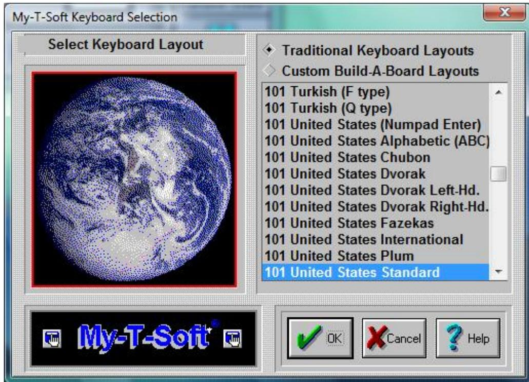
My-T-Soft TS can operate with many different keyboard layouts. By selecting the same keyboard layout that Windows uses, you can synchronize the display on My-T-Soft TS with the characters generated in your application.
