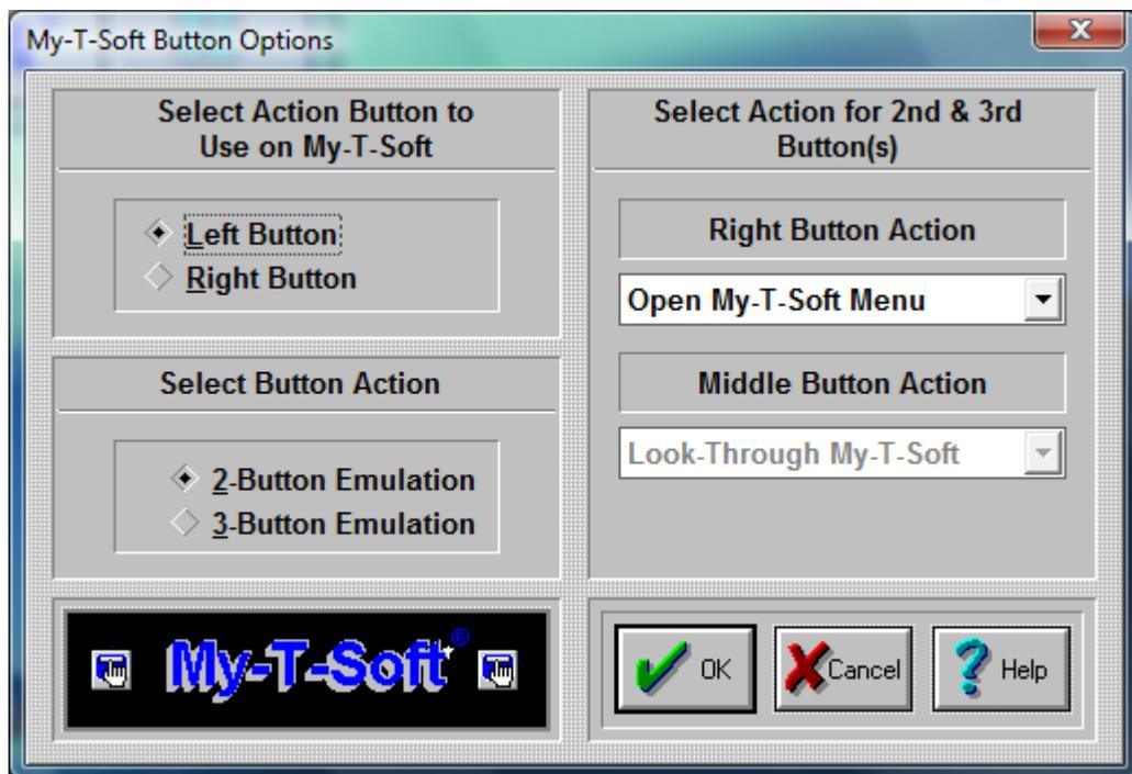
**Important:** The term Mouse is used generically for any pointing device that moves the cursor (mouse pointer) within Windows. For Pen and Touchscreen drivers, often only 1 button is available (Left Button): In all cases, the Left Button should be selected as the Action button.
