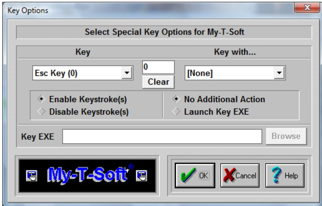
Key Options offers customization capabilities for keys on the main Alpha Keyboard Panel and the Edit panel. Keys may be disabled, assigned to other functions, and can be re-mapped using the Launch Key EXE in conjunction with the Developer's Kit (e.g. the Esc key could be re-mapped to send Alt-F4).
