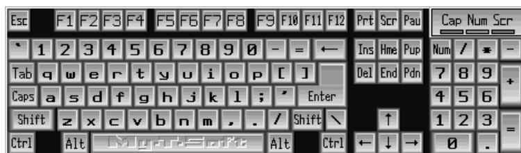
When you click any of the keys on the Keyboard (Alpha) Panel, Edit Panel, and Numeric Panel, they will respond exactly like the corresponding keystroke on a physical keyboard. In order to type with My-T-Soft TS, another window must be the Active Application and have the input focus. Windows typically indicate where typed characters will be displayed by the Caret, or text cursor. This usually is displayed as a flashing bar, although other shapes may be used.
