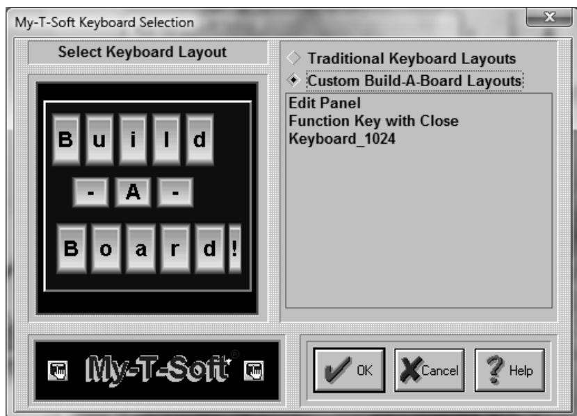
There are a few sample, custom Build-A-Board Layouts available. Additional Build-A-Board layouts can be created, and when placed in the Installation Folder will be added to this list. When selected, the KEYBOARD.KBF in the users configuration folder is replaced with the selected layout. When My-T-Soft TS is run, the layout is recognized, and the Build-A-Board compatible run-time (MYTSOFT2.EXE) is used to operate with the version 2.x keyboard layouts.
