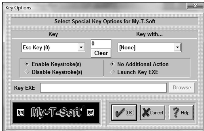
Key Options offers customization capabilities for keys on the main Alpha Keyboard Panel and the Edit panel. Keys may be disabled, assigned to other functions, and can be
