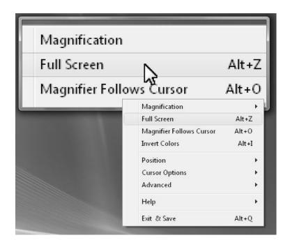
Full Screen When selected in the Windowed mode of operation, this will go to the Full Screen mode of operation. Keyboard Shortcut: Alt-Z. For further details on Full Screen operation, see the next chapter.
