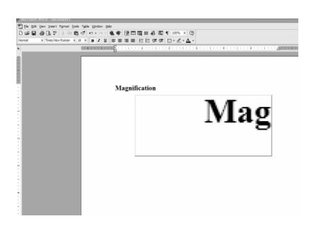
**4x Magnification** This selection will allow The Magnifier to show the image on your screen four times as large as they would normally appear. Keyboard Shortcut: **Alt-4**
