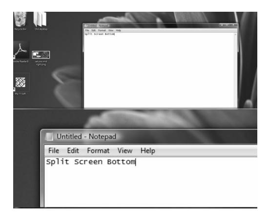
Split-Screen - Bottom This option will enlarge The Magnifier's window to the entire bottom portion of your screen. In order to utilize the items normally found on the bottom of your screen, you must drag The Magnifier's window using your left mouse button. The benefit to this
