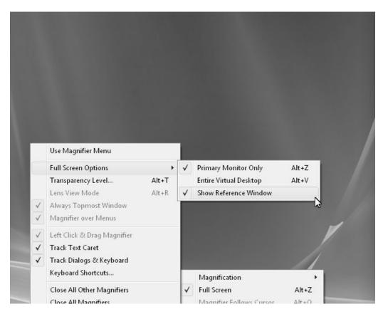
Primary Monitor Only This toggles the full screen mode of operation on the primary monitor (main display) Unless you have multiple monitors, this is the most common option. Keyboard Shortcut: Alt-Z
