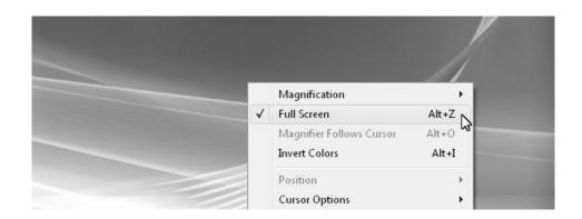
Full Screen When selected in the Full Screen mode of operation, this will clear this setting, and you will go to the Windowed mode of operation.
