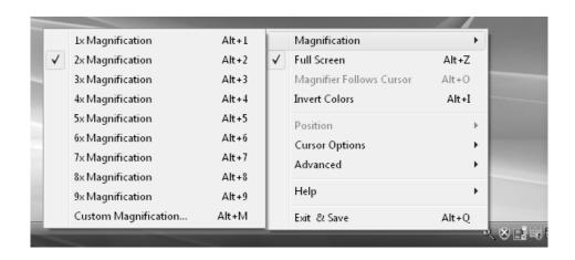
1x Magnification This selection does not change the image on your computer screen. By making this selection you will simply be able to view the screen without any magnification (exactly as it appears). In Full Screen mode, this is effectively the same as using Alt-S to hide The Magnifier window. Keyboard Shortcut: Alt-1
