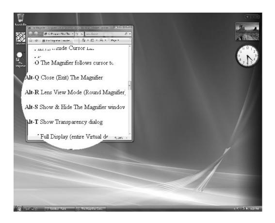
Lens View Mode This option transforms The Magnifier window into a circle (lens view). You can also toggle this mode with the keyboard shortcut Alt-R. The circle size is controlled by the shortest size (height or width) when going into lens view
