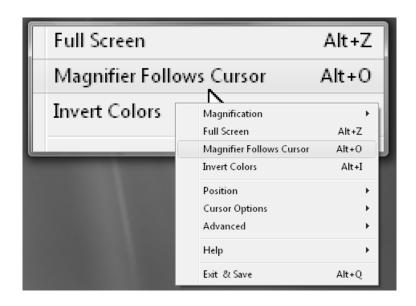
This option results in The Magnifier's window to follow the cursor as you move it across your screen. The position of The Magnifier window relative to the mouse cursor will change to make sure it is always visible on the screen. You can enable /
